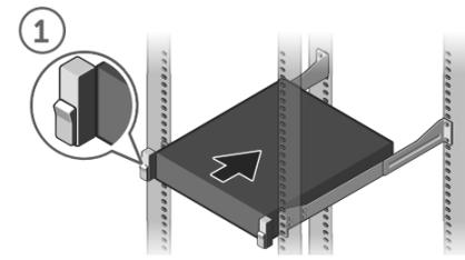
1 Install the system in to a rack.
